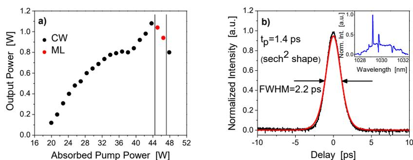
Figure 1: (a) Input-output characteristics of the laser in CW (black dots) and ML operation (red dots). (b) Autocorrelation curve (black line) and fit assuming sech<sup>2</sup> pulse shape (red line); optical spectrum (inset).
