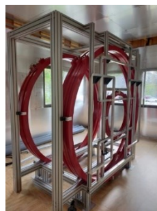
Fig.2: A photo of our MRI under construction. We see the coils generating the main B_0 field (in red) and the gradient coils placed on the outside of the main field coils (gray rectangles). The whole set-up is placed in a Faraday cage in order to limit the external noise.
